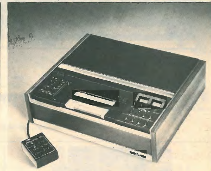
One of the current JVC range of 3/4 in. U-format video cassette recorders, with full remote control.
