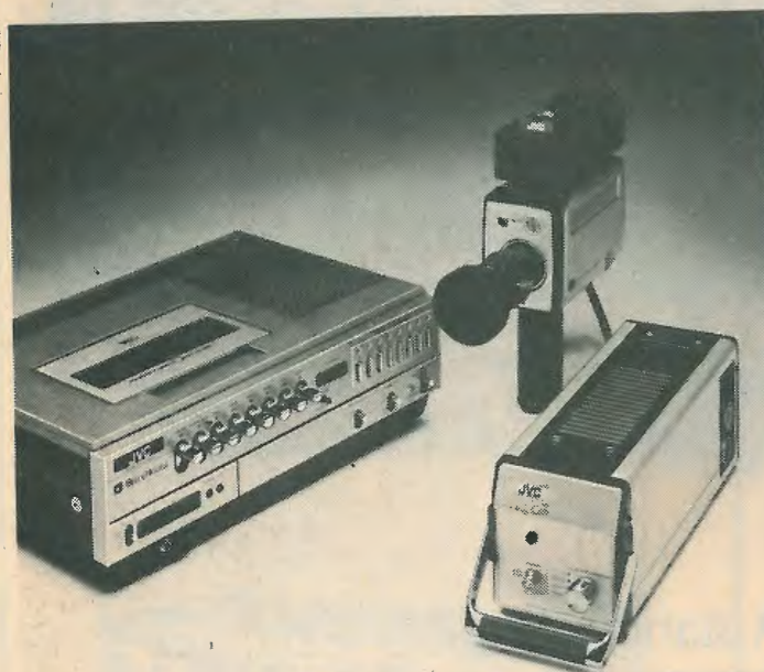
The JVC VHS recorder and GC3300 camera form an economical colour system for duties like rôle playing and product demonstrations.
